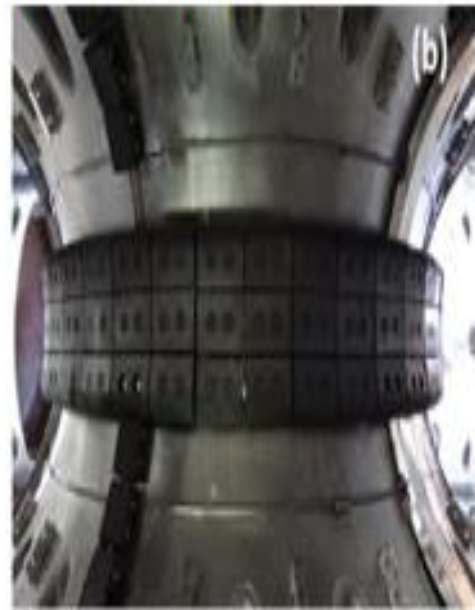
(a) Poloidal ring limiters. (b) Toroidal belt limiter
